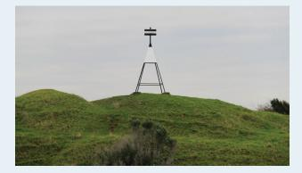
The structure that you can see sitting atop the summit is a 'Trig Beacon' - a geodetic survey mark (instrument used to measure the earth), it forms a component of New Zealand's geodetic system. It's one of a network of Trig Stations across New Zealand that serve as a physical reference point. They are used in the creation of maps, charts and interestingly they are essential to determining property boundaries.
